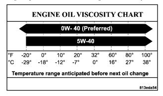
The engine oil filler cap also shows the recommended engine oil viscosity for your engine. For information on engine oil filler cap location, refer to "Engine Compartment" in this section.
